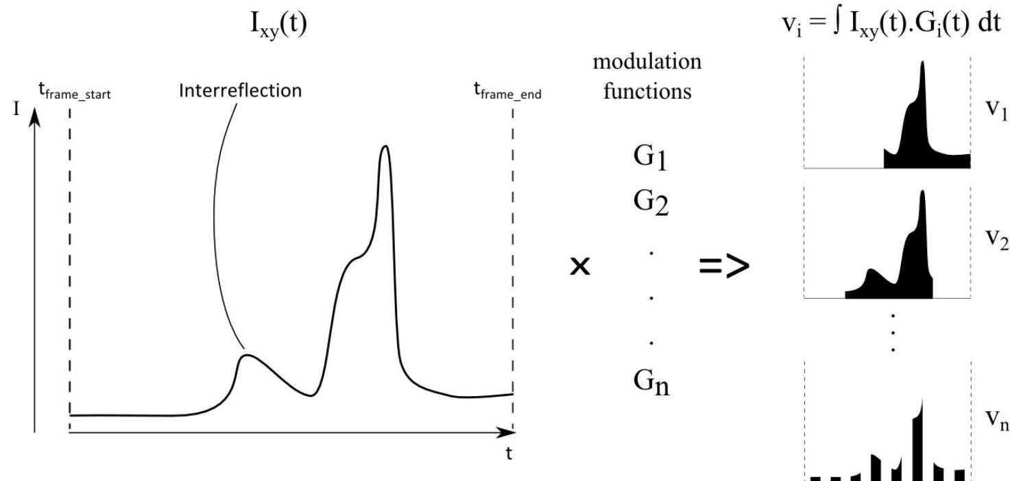
$$\text{accumulated value} = \int_{t_{frame\_start}}^{t_{frame\_end}} \text{incoming light}(t) \cdot \text{modulation signal}(t) dt$$
