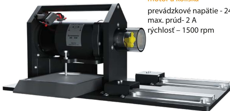
DC Dynamometer / motor a kolíska
